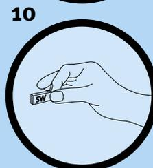
10 Refit jumper SW2 to exit programming.
